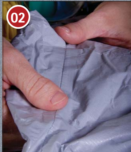
CAREFULLY INSPECT THE SEAMS OF THE SUIT FOR TEARS OR BROKEN SEALS
