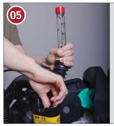
TEMPORARILY ATTACH BATTERY AND TEST PAPR MOTOR USING AIR FLOW METER
