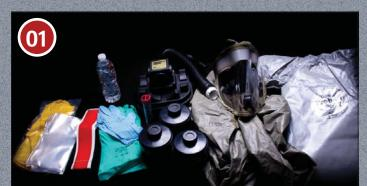
BATTERIES: YELLOW - RECHARGEABLE; WHITE - ONE TIME USE EQUIPMENT: PAPR AND HOOD, BATTERIES, FILTERS, DUCT TAPE, SUIT, INNER BOOTS, OUTER BOOTS, INNER GLOVES, OUTER GLOVES
