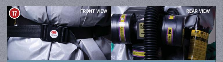
APPLY PAPR MOTOR AND BELT. CLIP BATTERY TO BELT. ATTACH BATTERY TO PAPR MOTOR
