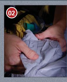
CAREFULLY INSPECT THE SEAMS OF THE SUIT FOR TEARS OR BROKEN SEALS
