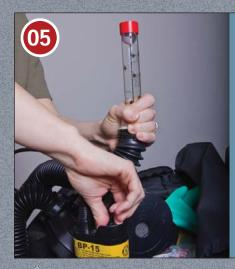
TEMPORARILY ATTACH BATTERY AND TEST PAPR MOTOR USING AIR FLOW METER
