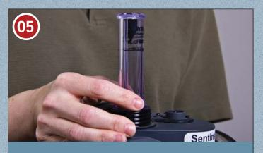
TEST PAPR MOTOR USING AIR FLOW METER
